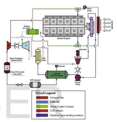
Fig. 8. Schematic view of the proposed layout of Rankine Cycle installation. Working media: steam
