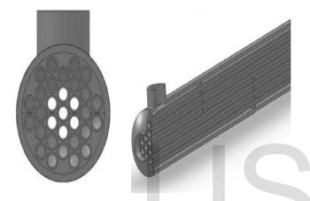
Fig. 4 Optomized Shell and tube Heat Exchanger.
